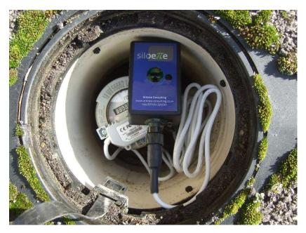
The logger records the flow through the meter at sub 1-second resolution. Once downloaded an algorithm is applied to the data to create a high-resolution flow trace of the flow into the property, as illustrated in Figure 4.
