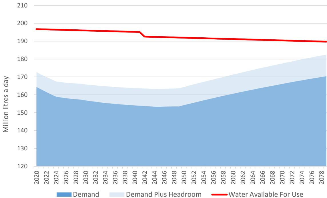
Figure 2: SES Water Final Supply Demand Balance (WRMP19)
